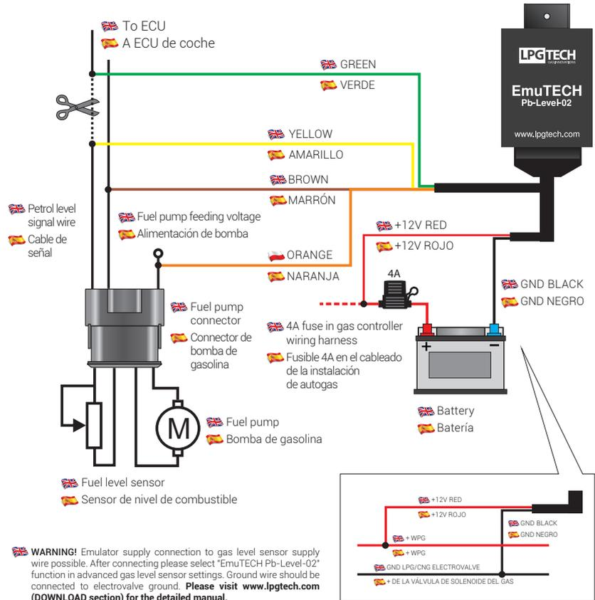
**🇬🇧 WARNING!** Emulator supply connection to gas level sensor supply wire possible. After connecting please select "EmuTECH Pb-Level-02" function in advanced gas level sensor settings. Ground wire should be connected to electrovalve ground. **Please visit [www.lpgtech.com](http://www.lpgtech.com) (DOWNLOAD section) for the detailed manual.**
