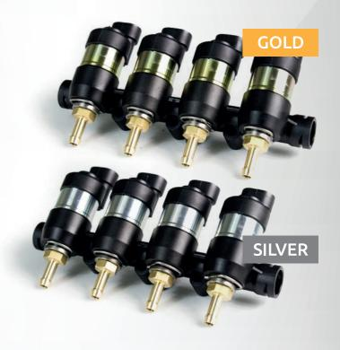
TECH-DRAGON is an injection rail of LPG/CNG volatile gas phase. It can be easily installed in hard to reach places under the bonnet because of small diameters. Application of fluoropolymer coating prevents the moving injector parts from sticking of contaminants. This allows faultless operation and precise gas dosage. Reduction of friction significantly extends injector lifespan.
