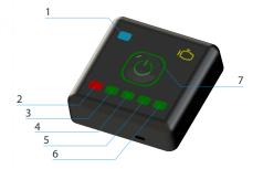
The microprocessor controller TECH is responsible for correct operation of the autogas system in the vehicle, as it collects all data on the engine work and gas pressure and temperature, and controls other parameters of the system.
